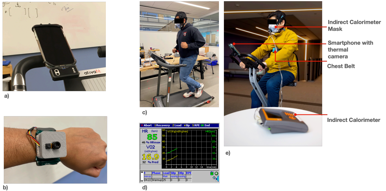
Fig. 4. JoulesEye’s is composed of a thermal camera retrofitted in an iPhone as shown in a) . JoulesEye can be used in a smartwatch as shown in b) . The camera in b) is a low resolution (32x24) thermal camera. c) and e) show the ground truth data collection procedure with indirect calorimeter while running and biking. d) shows a screen grab from the indirect calorimeter recording the energy expenditure during an exercise session.
