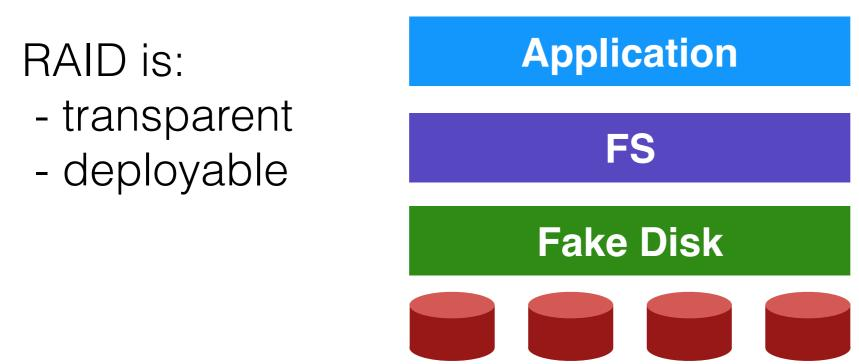
RAID: Redundant Array of Inexpensive Disks
