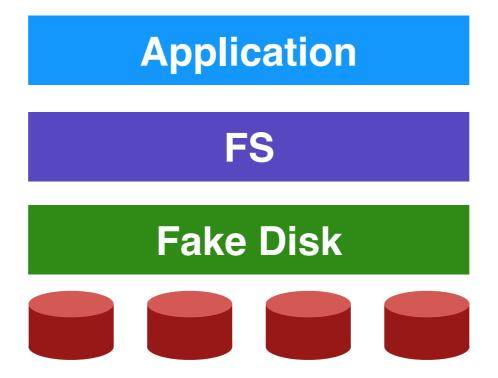
RAID: Redundant Array of Inexpensive Disks
