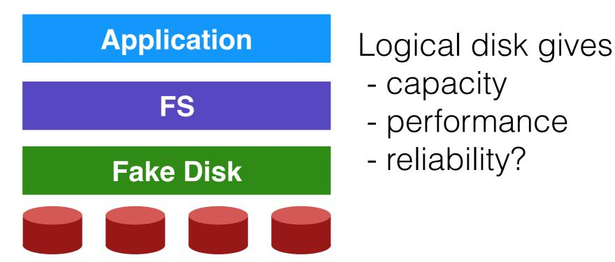
RAID: Redundant Array of Inexpensive Disks
